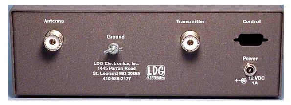
"What's the deal with the hole?" Sharp-eyed users will note an empty cutout labeled "Control" on the back panel. Future versions of the AT-1000 may feature remote control and monitoring via a DB-9 connector in this position. This feature may also be offered as an upgrade for present users, but is not available at this time. In this version, the cutout serves no function. Never insert anything into this cutout, especially when transmitting.
