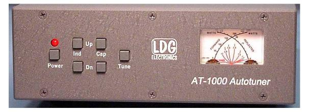
The Power switch does not turn the tuner completely off. It places it in a low-current "sleep" mode. In the Off mode, the tuner is in bypass, routing RF directly from your amplifier to the antenna with no matching. On power-up, the tuner is automatically restored to the last tuned setting. If DC power is interrupted, the tuner will revert to bypass mode on power-up.
