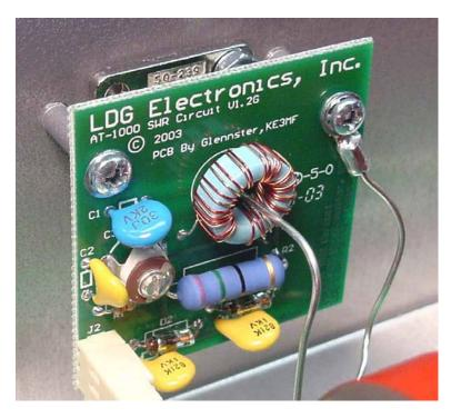
The relays operate from an external 12 volt DC power supply. The total current drawn by the AT-1000 depends primarily on the number of energized relays, with the maximum current drain being approximately 1 Amp. The microprocessor also needs a power supervisory circuit (U2, the 34064 IC) to provide a proper power-on sequence and to place the microprocessor in a known reset mode while powering down.
