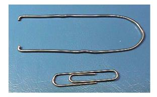
The extraction tool fits into opposite corners of the 68HC11 socket; the bent ends will lift the chip from beneath. Unplug the tuner, touch a ground point to avoid static discharge damage, and remove the cabinet cover. Insert the tool and pull gently and evenly on both sides to extract the chip. Press the upgrade chip into the socket, observing the small diagonal corner key. Replace the cabinet cover; your upgraded AT-1000 is ready to use.
